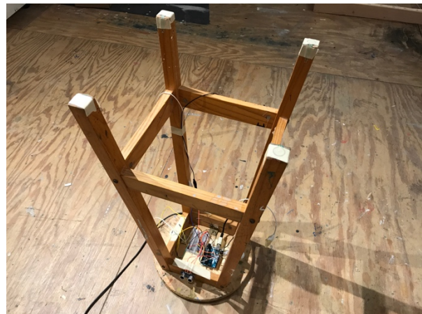
Figure 4. Stool including pressure sensors on the feet, an array of motion detectors and proximity sensors on each side, and a vibration motor on the stool top.
