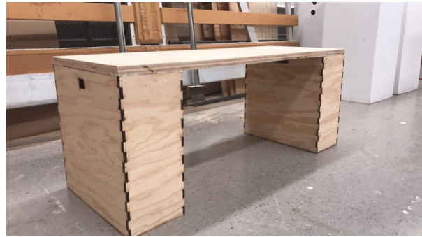
Figure 6. Laser cut bench prototype with specific slots for proximity sensors and wiring. Width of the legs is wide enough for motors and wheels.
